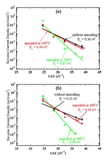
FIG. 6. Relationship of the reverse-bis current measured at -3 V for (a)  $n^+$ -*Si/n-SiC* and (b)  $p^+$ -*Si/n-SiC* junctions without being annealed and annealed at 400 and 700 °C.
