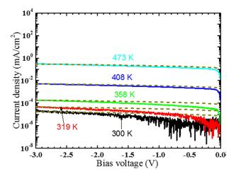
FIG. 7. Reverse *I-V* characteristics of  $n^+$ -*Si/n-SiC* junctions annealed at 700 °C measured at various temperatures. The fitting curves using the thermionic-field emission theory are shown by a dotted line.
