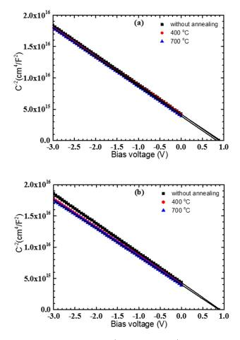
FIG. 2. *C-V* characteristics of (a)  $n^+$ -*Si/n-SiC* and (b)  $p^+$ -*Si/n-SiC* junctions without being annealed and annealed at 400 and 700 °C measured at room temperature.
