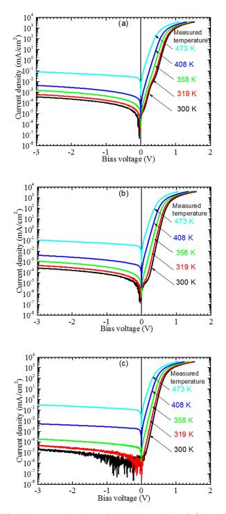
FIG. 4. Temperature dependence of the *I-V* characteristics of  $p^+$ -*Si/n-SiC* junctions (a) without being annealed (Reprinted with permission from Appl. Phys. Lett. **104**, 161604 (2014). Copyright 2014 AIP Publishing LLC) and annealed at (b) 400 and (c) 700 °C measured at various temperatures.
