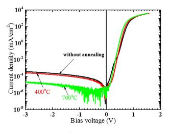
FIG. 1. *I-V* characteristics of  $n^+$ -*Si/n-SiC* junctions without being annealed and annealed at 400 and 700 °C measured at room temperature.
