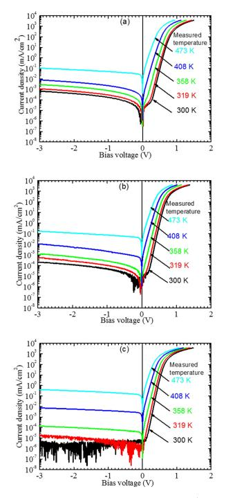
FIG. 3. Temperature dependence of the *I-V* characteristics of  $n^+$ -*Si/n-SiC* junctions (a) without being annealed (Reprinted with permission from Appl. Phys. Lett. **105**, 151607 (2014). Copyright 2014 AIP Publishing LLC) and annealed at (b) 400 and (c) 700 °C measured at various temperatures.
