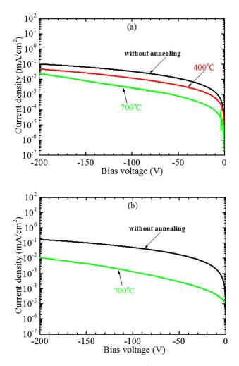
FIG. 5. Reverse *I-V* characteristics of (a)  $n^+$ -*Si/n-SiC* junctions without being annealed and annealed at 400 and 700 °C and (b)  $p^+$ -*Si/n-SiC* heterojunctions without being annealed and annealed at 700 °C.
