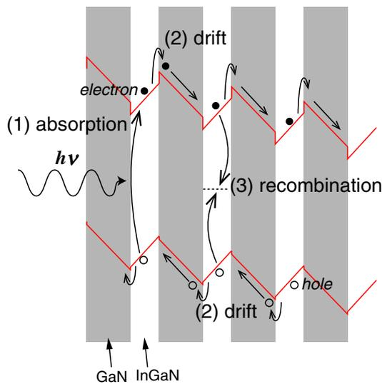
**Fig. 12.** (Color online) Schematic plots of band profiles and the elementary process of the solar cell operation in the MQW structure: (a) photon absorption in the well layer, (b) transport of the photoinduced carrier in the barrier layer (drift), and (c) carrier disappearance through nonradiative recombination process.
