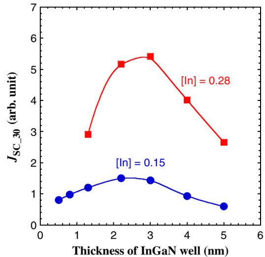
**Fig. 15.** (Color online) Calculated short-circuit current of 30-period-MQW solar cell as a function of the thickness of the InGaN well layer.
