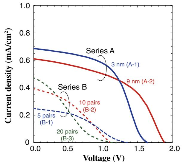
**Fig. 2.** (Color online)  $J$ - $V$  curves of InGaN/GaN MQW solar cells under AM 1.5 G illumination.
