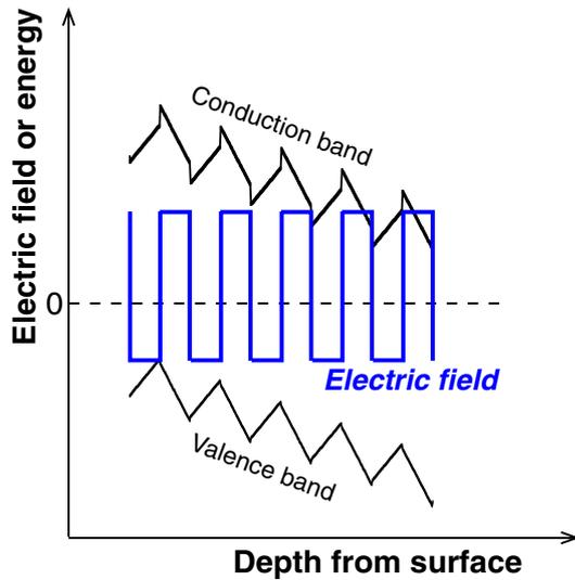
**Fig. 7.** (Color online) Schematic plots of band profiles and internal electric field for MQW structure.
