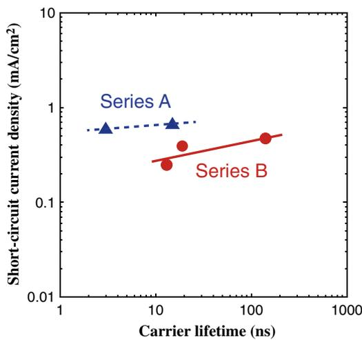
**Fig. 5.** (Color online) Carrier lifetime dependence of short-circuit current density.
