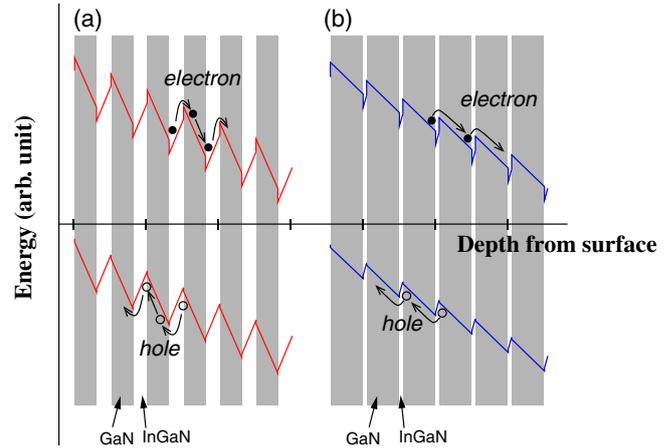
**Fig. 13.** (Color online) Schematic plots of band profiles of MQW with (a)  $w_B \approx w_W$  and (b)  $w_W \ll w_B$ .
