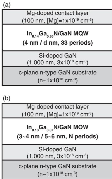
**Fig. 1.** Epitaxial layer structures of solar cells with InGaN/GaN MQW absorption layers. (a) Series A: different barrier thicknesses (3 and 9 nm), the same well thickness, and the same number of InGaN well layers. (b) Series B: different numbers of wells (5, 10, and 20 pairs) and the same InGaN/GaN unit QW layers.
