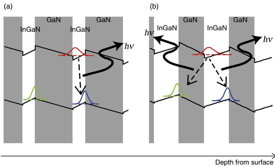
**Fig. 4.** (Color online) Schematic band profiles of the InGaN/GaN MQWs with different barrier and well layer thicknesses and wave functions of electrons in the conduction band and holes in the valence band: (a)  $d_{\text{InGaN}} < d_{\text{GaN}}$  and (b)  $d_{\text{InGaN}} \approx d_{\text{GaN}}$ .
