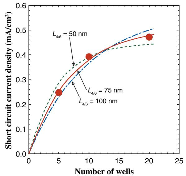
**Fig. 8.** (Color online) Short-circuit current density of series-B samples as a function of the number of well layers in InGaN/GaN MQW. Curves show results calculated using Eq. (4) with various specific lengths.
