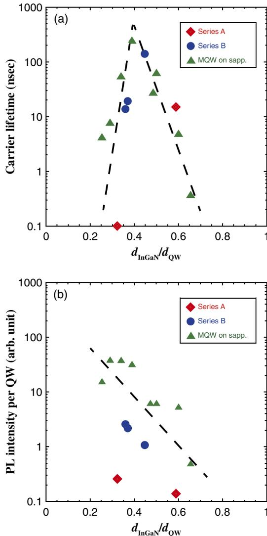
**Fig. 3.** (Color online) MQW structure dependence of (a) the lifetime of photoinduced carriers estimated from TRPL and (b) the PL intensity per QW. Broken lines are guides for the eyes.
