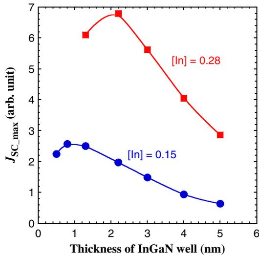
**Fig. 14.** (Color online) Calculated maximum short-circuit current of InGaN/GaN MQW solar cell as a function of the thickness of the InGaN well layer.
