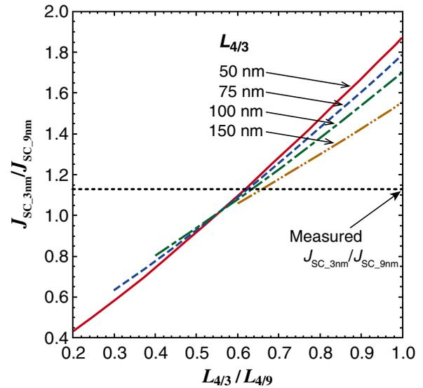
**Fig. 10.** (Color online) Specific length of the MQW solar cells from this work, Ref. 30, and Ref. 34 as a function of the ratio of InGaN well thickness to the GaN barrier thickness.
