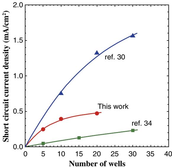
**Fig. 9.** (Color online) Dependence of short-circuit current density on the number of wells in InGaN/GaN MQW for samples in our series B, Refs. 30 and 34.
