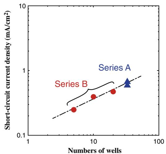
**Fig. 6.** (Color online) Dependence of short-circuit current density on the number of wells in InGaN/GaN MQW.
