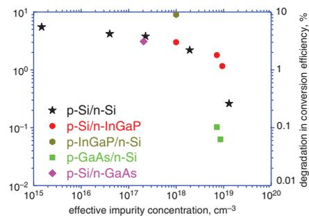
**Fig. 2** Power loss and degradation in conversion efficiency against effective impurity concentrations in  $p$ -Si/ $n$ -Si,  $p$ -Si/ $n$ -InGaP,  $p$ -InGaP/ $n$ -Si,  $p$ -GaAs/ $n$ -Si, and  $p$ -Si/ $n$ -GaAs junctions
