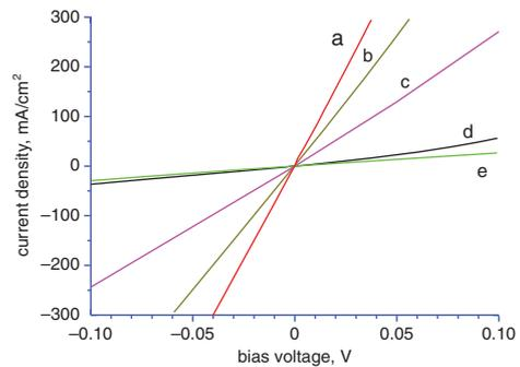
**Fig. 1**  $I$ - $V$  characteristics of (a)  $p^+$ -GaAs/ $n^{++}$ -Si; (b)  $p^+$ -GaAs/ $n^+$ -Si; (c)  $p^+$ -Si/ $n^+$ -Si; (d)  $p^{++}$ -Si/ $n^+$ -InGaP; and (e)  $p^+$ -Si/ $n^+$ -InGaP junctions measured at room temperature
