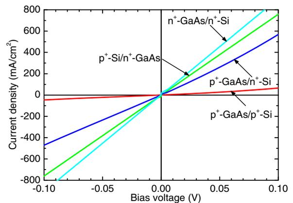
Fig. 2. (Color online) *I*-*V* characteristics of p<sup>+</sup>-GaAs/p<sup>+</sup>-Si, p<sup>+</sup>-Si/n<sup>+</sup>-GaAs, p<sup>+</sup>-GaAs/n<sup>+</sup>-Si, and n<sup>+</sup>-GaAs/n<sup>+</sup>-Si junctions measured at room temperature.
