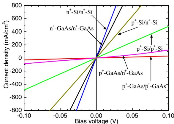
**Fig. 4.** (Color online)  $I$ - $V$  characteristics of  $n^+$ -Si/ $n^+$ -Si,  $p^+$ -Si/ $n^+$ -Si,  $p^+$ -Si/ $p^+$ -Si,  $n^+$ -GaAs/ $n^+$ -GaAs,  $p^+$ -GaAs/ $n^+$ -GaAs, and  $p^+$ -GaAs/ $p^+$ -GaAs junctions measured at room temperature.
