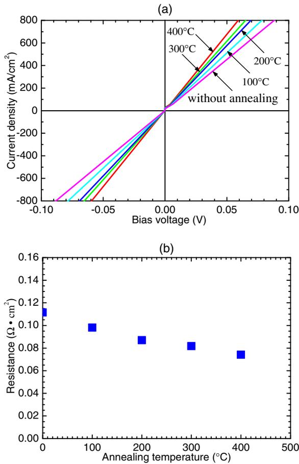
**Fig. 3.** (Color online) (a)  $I$ - $V$  characteristics of  $n^+$ -Si/ $n^+$ -GaAs junctions without and with annealing at 100, 200, 300, and 400 °C measured at room temperature and (b) resistances of the respective samples at various annealing temperatures for  $n^+$ -Si/ $n^+$ -GaAs junctions.
