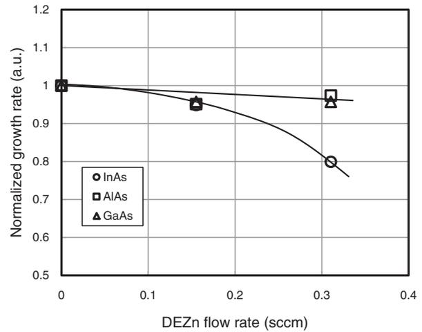
**Fig. 6.** Normalized growth rate of InAs, AlAs, and GaAs components as a function of DEZn flow rate.
