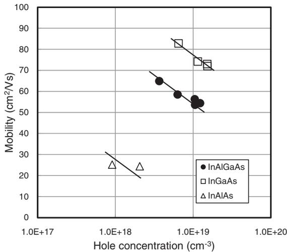
**Fig. 2.** Relationship between mobility and hole concentration in Zn-doped InGaAs, Zn-doped InAlAs, and Zn-doped InAlGaAs layers.
