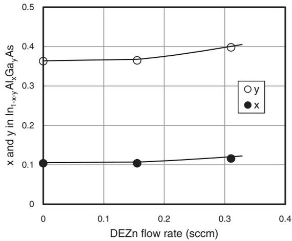
**Fig. 5.** The  $x$  and  $y$  in Zn-doped  $\text{In}_{1-x-y}\text{Al}_x\text{Ga}_y\text{As}$  layer as a function of DEZn flow rate.
