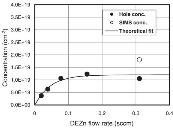
**Fig. 1.** Hole and Zn concentration as a function of DEZn flow rate. Closed circles and the open circle indicate the hole concentration and Zn concentration, respectively. The solid curve is a theoretical fit using eq. (8).
