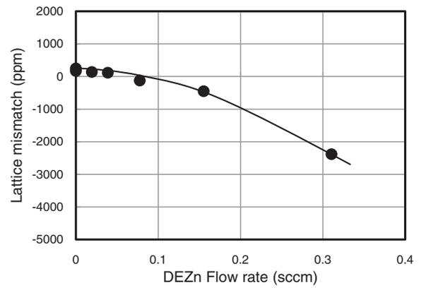
**Fig. 3.** Relationship between lattice mismatch and DEZn flow rate in Zn-doped InAlGaAs layers.
