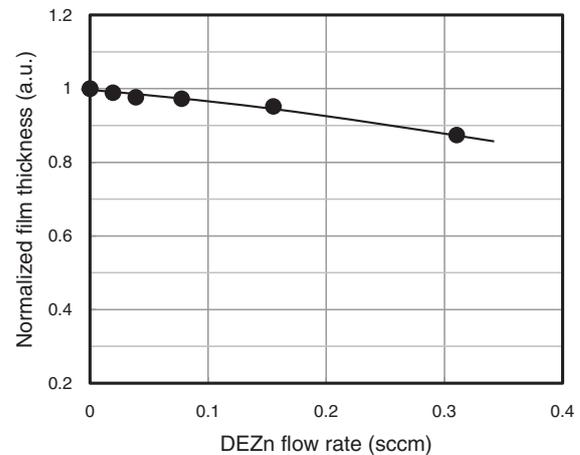
**Fig. 4.** Normalized film thickness of the InAlGaAs layer as a function of DEZn flow rate.
