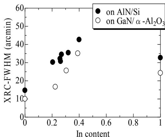
**Figure 4** XRC-FWHM in InGaN films grown on AlN/Si (111) and GaN/ $\alpha$ -Al<sub>2</sub>O<sub>3</sub> (0001) substrates as a function of In content.
