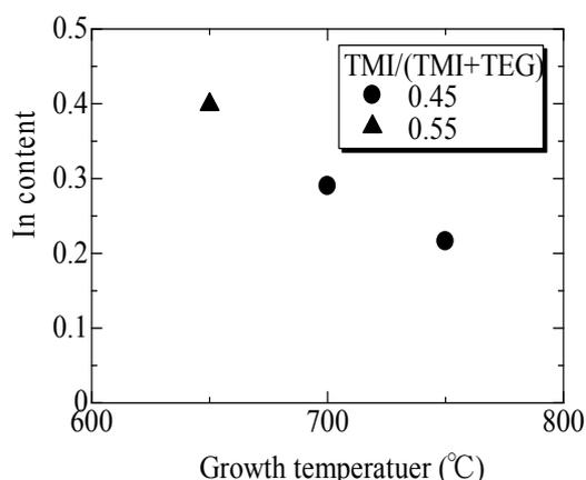
**Figure 3** In content in InGaN films as a function of growth temperature as a parameter of TMI/(TMI+TEG) molar ratio.
