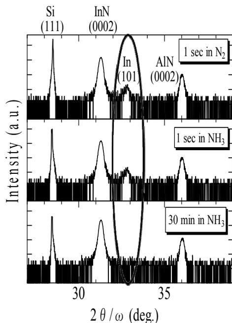
**Figure 1** XRD  $2\theta/\omega$  profiles of InN films grown on AlN/Si(111) substrate with different substrate pretreatments at 1000 °C.
