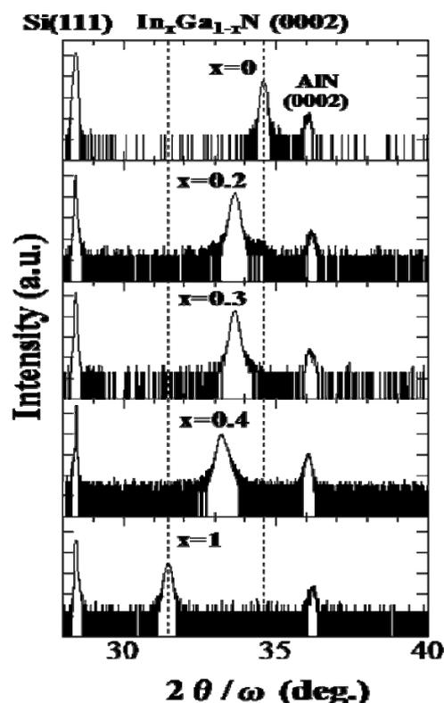
**Figure 2** XRD  $2\theta/\omega$  profiles of  $\text{In}_x\text{Ga}_{1-x}\text{N}$  films grown on AlN/Si(111) substrate with different In contents.
