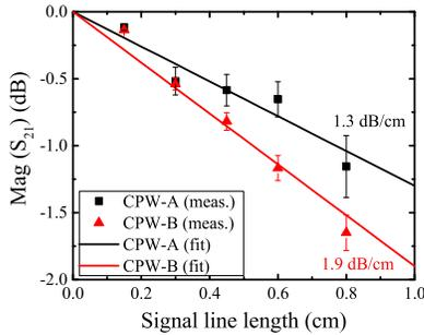
Fig. 6. Relationships between the insertion loss and the length for the two types of CPWs at 20 GHz.
