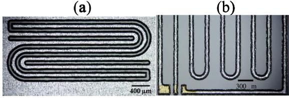
Fig. 3. Top view of (a) 8-mm-long meander-shaped CPW-A and (b) IND-A with  $n = 3$  and  $d = 200 \mu\text{m}$ . (a) Its  $W$  and  $S$  were  $90 \pm 20$  and  $60 \pm 20 \mu\text{m}$  and (b)  $W$  and  $d$  were  $90 \pm 20$  and  $210 \pm 20 \mu\text{m}$ , respectively.
