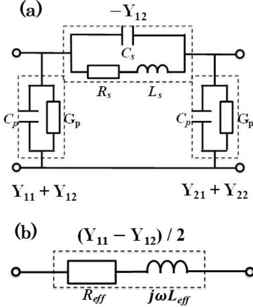
Fig. 4. (a)  $\pi$ -type equivalent circuit of two-port INDs. (b) Model of the conductance along the signal lines of INDs.
