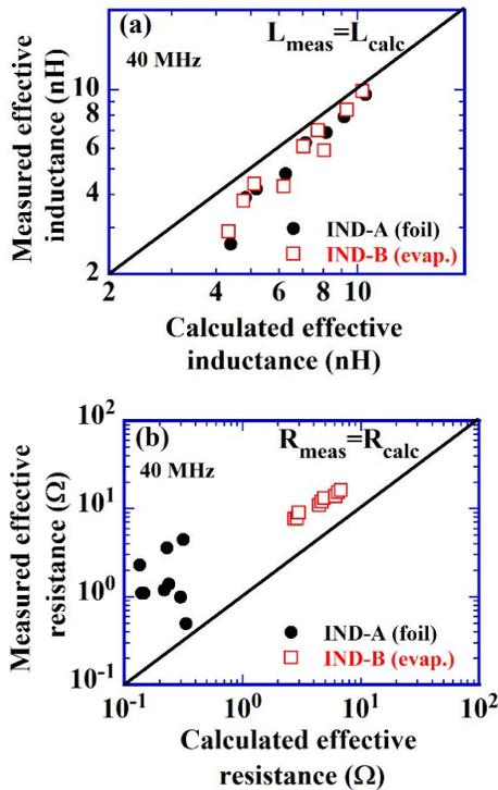
Fig. 9. Relationships between (a) measured and calculated  $L_{\text{eff}}$  at 40 MHz and (b) measured and calculated  $R_{\text{eff}}$  at 40 MHz. Guides for eyes are also shown.
