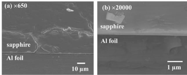
Fig. 1. Field-emission scanning electron microscope image of a bonding interface of an Al-foil/sapphire junction with a magnification scale of (a) 650 $\times$  and (b) 20 000 $\times$ .
