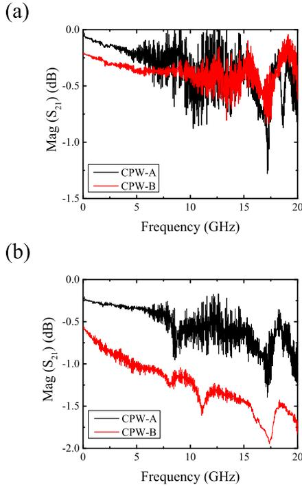
Fig. 5. Transmission characteristics for (a) 3-mm CPWs and (b) 8-mm CPWs, respectively.
