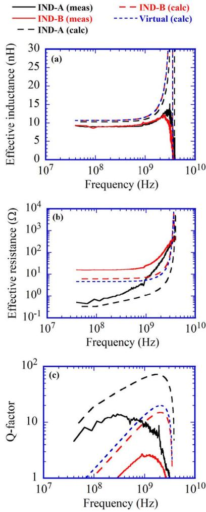
Fig. 8. Measured and calculated (a) effective inductances, (b) effective resistances, and (c)  $Q$ -factors for INDs with  $n = 3$  and  $d = 300 \mu\text{m}$ .
