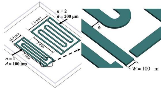
Fig. 2. Geometries of INDs with  $n = 1$ ,  $d = 100 \mu\text{m}$  and  $n = 2$ ,  $d = 200 \mu\text{m}$ .
