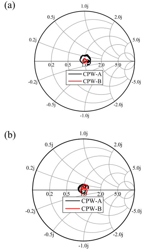
Fig. 7. Return loss characteristics for (a) 3-mm CPWs and (b) 8-mm CPWs, respectively.
