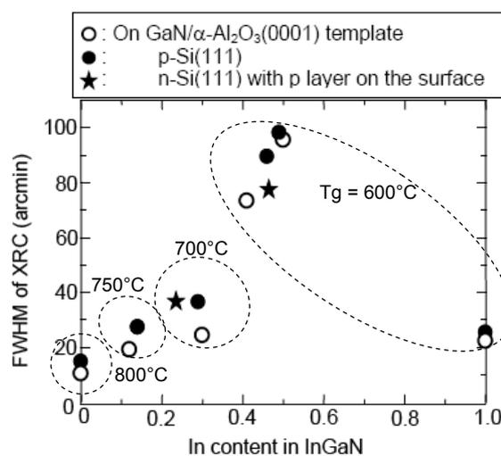
**Figure 3** In composition dependence of FWHM of X-ray rocking curve, tilt fluctuation, for InGaN films grown on different substrates at a different temperature  $T_g$ .
