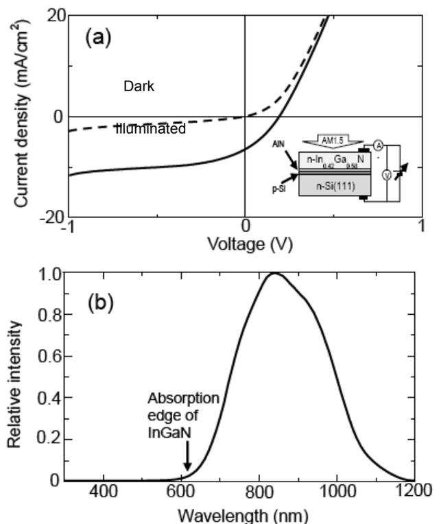
**Figure 5** I-V characteristics (a) and spectral response (b) for n-In<sub>0.42</sub>Ga<sub>0.58</sub>N/pn-Si structure. The inset in (a) shows the schematic cross-sectional view of the sample.
