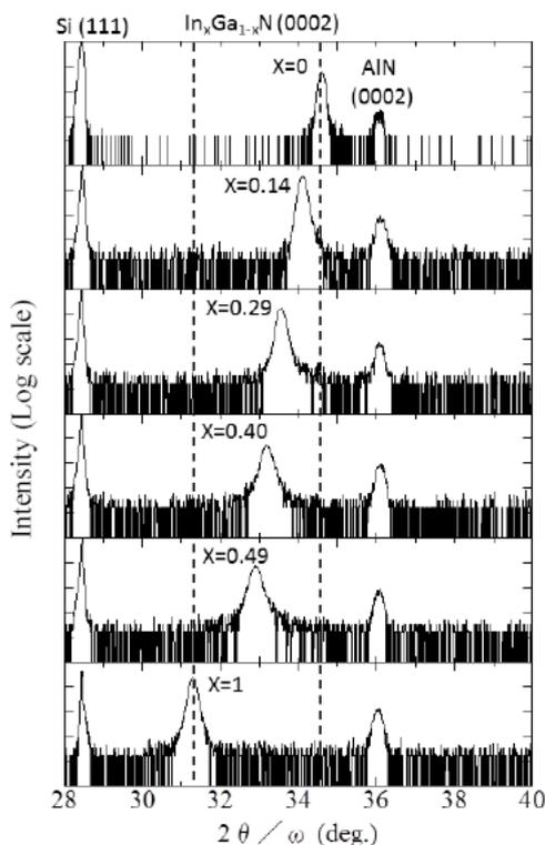
**Figure 1** X-ray diffraction (XRD)  $2\theta/\omega$  profiles for InGaN films with a different In composition grown on Si(111) substrates. A 100 nm-thick AlN is used as an interlayer.
