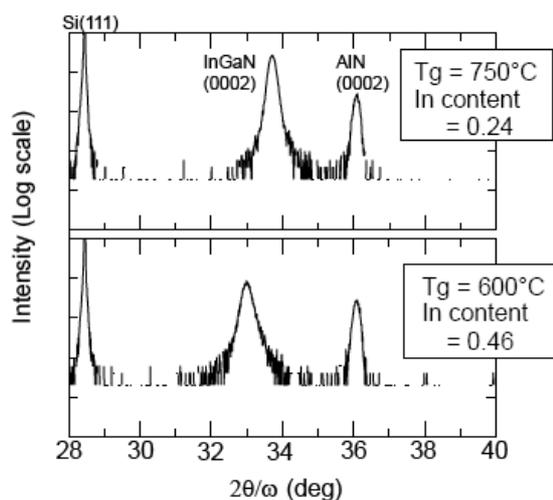
**Figure 2** XRD  $2\theta/\omega$  profiles for InGaN films grown on n-Si(111) substrates with a p layer on the surface. Two films with a different In composition are grown with a constant TMI/(TMI+TEG) molar ratio 0.5 at a different temperature  $T_g$ .
