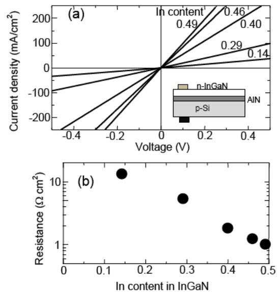
**Figure 4** I-V characteristics (a) and resistance (b) between n-InGaN and p-Si. The inset in (a) shows the schematic cross-sectional view of the measured sample.
