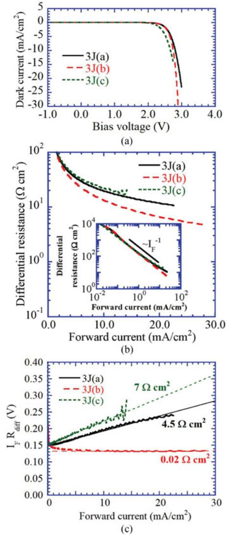
Fig. 4. (a)  $I$ - $V$  characteristics of the 3J cells in the dark. (b) Relationships between the differential resistance and forward current of the 3J cells in the dark. The inset shows the relationships on a log-log scale. (c) Dependence of the product of the forward current and differential resistance on the forward current.
