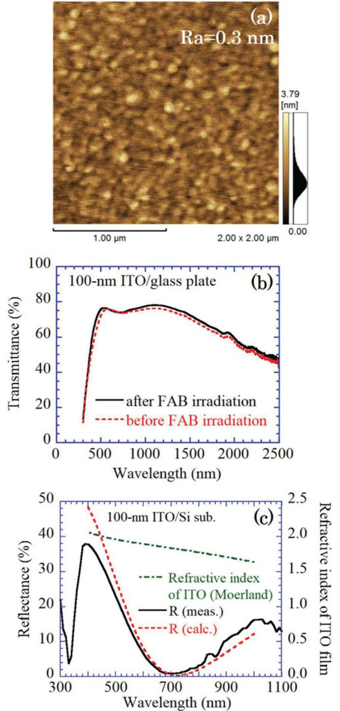
Fig. 2. (a) AFM image of an ITO film deposited on an Si substrate. (b) Optical transmittance spectra of a 100-nm-thick ITO film deposited on a glass plate. The spectrum measured after the Ar-beam irradiation is compared with that before irradiation. (c) Reflectance spectrum of a 100-nm-thick ITO film deposited on an Si (100) substrate. A comparison with a calculation using a reported refractive index of ITO [50] is also shown.
