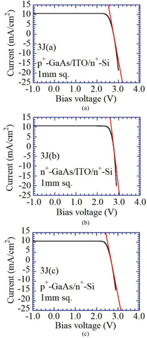
Fig. 6.  $I$ - $V$  characteristics of (a) 3J(a), (b) 3J(b), and (c) 3J(c) cells measured under solar irradiance of AM1.5G and one sun using in-house facilities. Red straight lines show the slopes at  $0 \text{ mA/cm}^2$  for the respective characteristics. The Si peripheries were not masked during the measurements.
