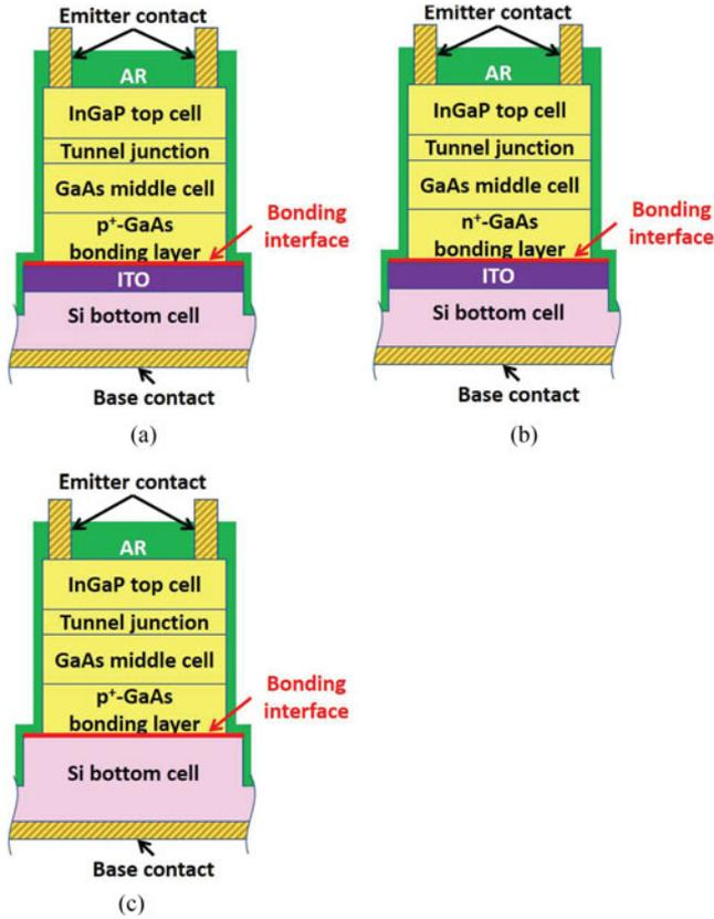
Fig. 1. Schematic cross-sections of (a) InGaP/GaAs/ITO/Si 3J cells with  $p^+$ -GaAs/ITO bonding interfaces [3J(a)], (b) InGaP/GaAs/ITO/Si 3J cells with  $n^+$ -GaAs/ITO bonding interfaces [3J(b)], and (c) InGaP/GaAs/Si 3J cells with  $p^+$ -GaAs/ $n^+$ -Si bonding interfaces [3J(c)].
