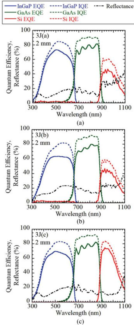
Fig. 5. Spectral responses of  $2 \times 2$ -mm (a) 3J(a), (b) 3J(b), and (c) 3J(c) cells. The external quantum efficiencies, reflectance, and internal quantum efficiencies are shown.
