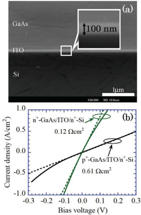
Fig. 3. (a) SEM image of a GaAs/ITO/Si junction. (b)  $I$ - $V$  characteristics of  $p^+$ -GaAs/ITO/ $n^+$ -Si and  $n^+$ -GaAs/ITO/ $n^+$ -Si two-terminal devices after annealing at 400 °C for 5 min. The differential resistances, or the slopes of the respective  $I$ - $V$  curves in the vicinity of 0 V, were estimated by using a least-squares fitting. The results of the fitting are shown by dashed lines.
