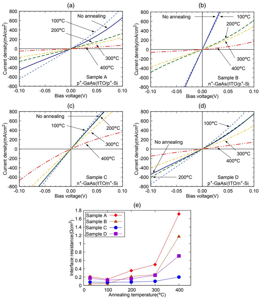
**Fig. 6.** (Color online)  $I$ - $V$  characteristics of Samples (a) A, (b) B, (c) C, and (d) D with annealing at different temperatures measured at room temperature and (e) resistance of the respective samples as a function of annealing temperature.
