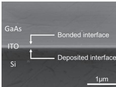
**Fig. 4.** Cross-sectional FE-SEM image of GaAs//ITO/Si interface.
