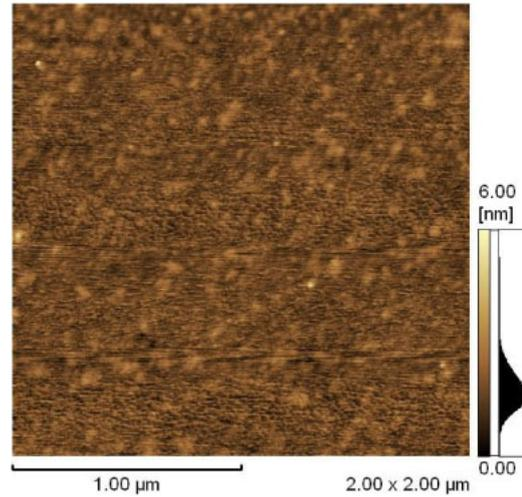
**Fig. 1.** (Color online) AFM image of surface of ITO film on Si substrate.
