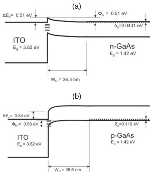
**Fig. 8.** Schematic energy-band diagrams of (a) ITO/n-GaAs and (b) ITO/p-GaAs interfaces.
