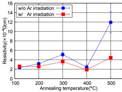
**Fig. 3.** (Color online) Resistance of ITO films without and with Ar irradiation as a function of annealing temperature. The error bars represent the  $1\sigma$  standard deviation of the mean.
