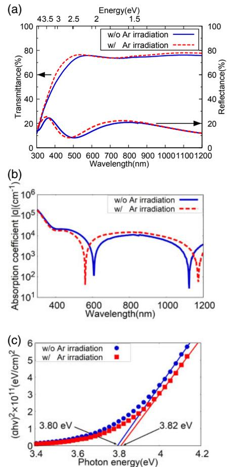
**Fig. 2.** (Color online) (a) Transmittance and reflectance of ITO film on glass plates, (b) absorption coefficient of ITO films calculated from transmittance and reflectance of respective samples, and (c) optical band gap energy of ITO films without and with Ar irradiation.
