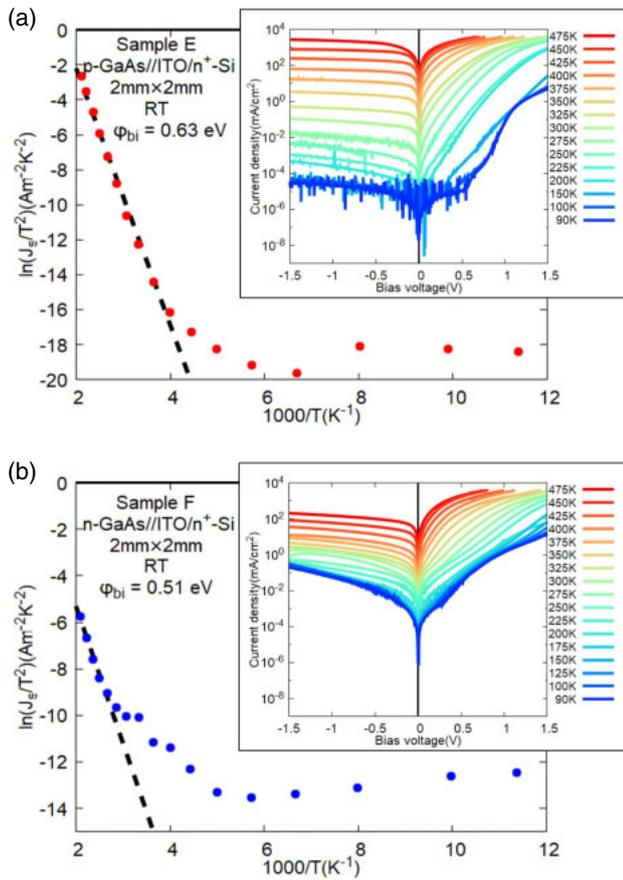
**Fig. 7.** (Color online) Arrhenius plot of  $\ln(J_s/T^2)$  versus  $10^3/T$  showing the temperature dependence of thermionic emission current in samples (a) E and (b) F. The inset shows the  $I$ - $V$  characteristics of the respective samples measured at temperatures between 90 and 475 K.
