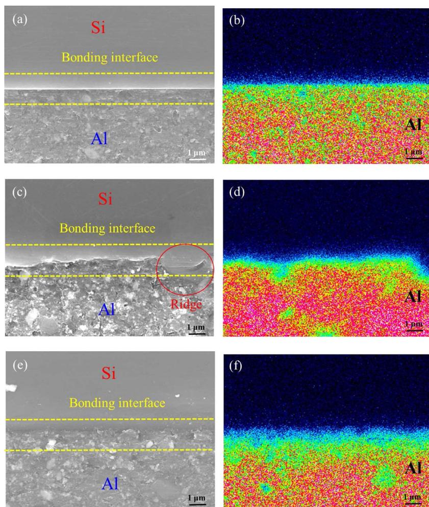
**Figure 9.** Cross-sectional FE-SEM images of the bonded Al/Si interfaces (a) without and with annealing at 1000°C for (c) 1 min and (e) 10 min. Results of the SEM/EDX-based elemental mapping of (b), (d), and (f) for (a), (c), and (e), respectively, for element Al.
