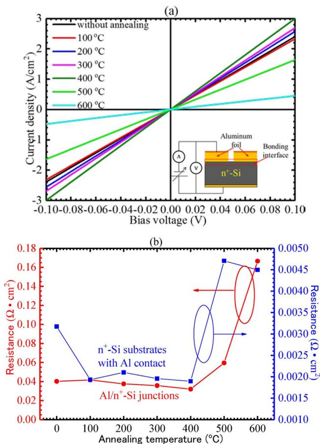
**Figure 7.** (a)  $I$ - $V$  characteristics of the bonded  $\text{Al}/n^+\text{-Si}$  junctions without and with annealing at various temperatures measured at room temperature and (b) the contact resistances of the bonded  $\text{Al}/n^+\text{-Si}$  junctions and the contact resistances of the evaporated Al electrode on  $n^+\text{-Si}$  substrates as a function of the annealing temperature.
