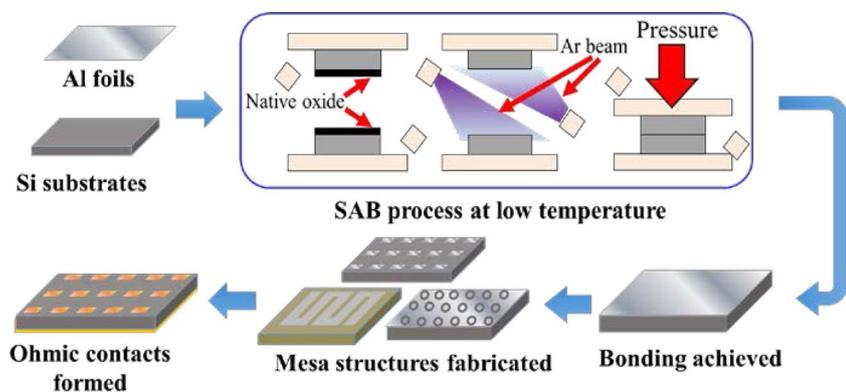
**Figure 1.** The fabrication processes of Al/Si junctions and Al structures on Si substrates.
