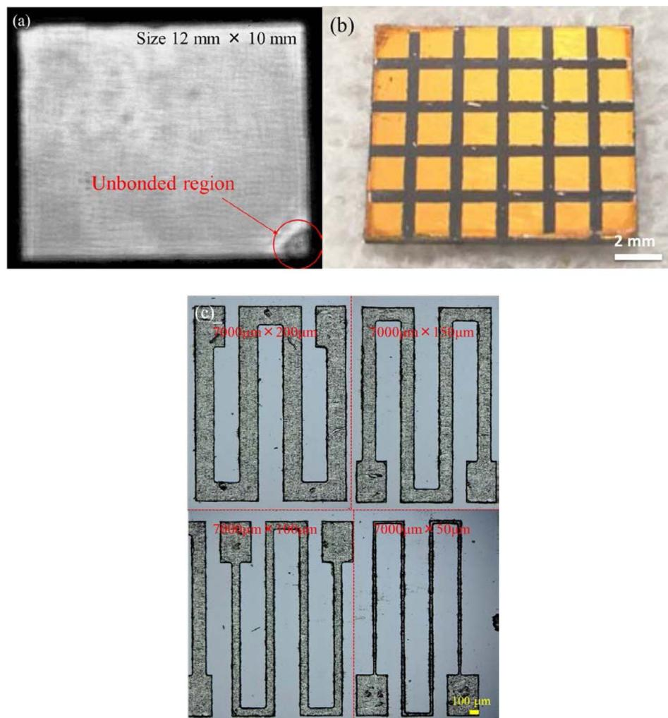
**Figure 2.** (a) A scanning acoustic microscopy image of Al/Si bonded sample, (b) Photograph of Al foil mesa-structures fabricated on Si substrates, and (c) Photograph of Al foil micro wiring with the length of 7000  $\mu\text{m}$  and the width of 200, 150, 100, 50  $\mu\text{m}$  fabricated on Si substrates.
