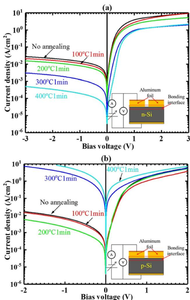
**Figure 5.**  $I$ - $V$  characteristics of the bonded (a) Al/ $n$ -Si and (b) Al/ $p$ -Si junctions without and with annealing at various temperatures measured at room temperature. The inset shows the schematic diagram of measurement.
