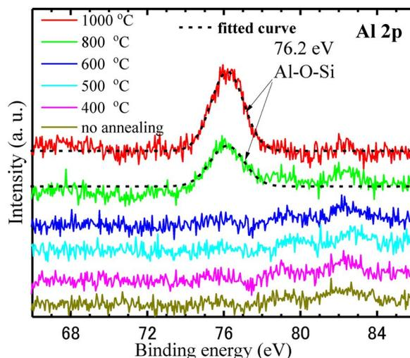
**Figure 8.** Al 2p photoemission spectra of Si substrates that were prepared by annealing the bonded Al/Si junctions at various temperatures and removing Al layer by wet etching.
