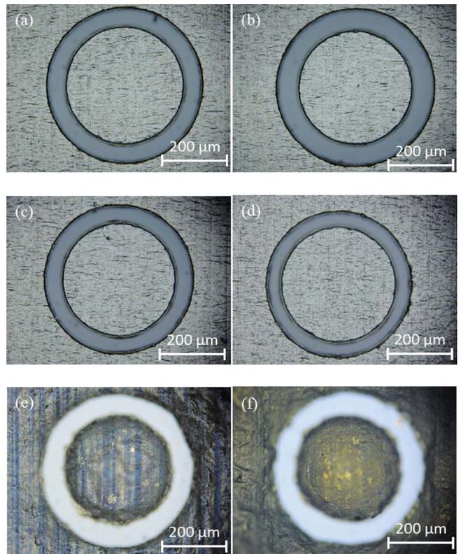
**Figure 4.** Photographs of Al circular mesa structures fabricated on Si substrate (a) without and with annealing at (b) 400, (c) 500, (d) 600, (e) 800, and (f) 1000°C.
