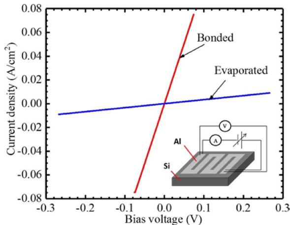
**Figure 3.** *I-V* characteristics of Al micro wiring with the length of 7000  $\mu\text{m}$  and the width of 200  $\mu\text{m}$  fabricated on Si substrate by evaporating and bonding. The thickness of the micro wiring fabricated by evaporating and bonding is 0.2 and 17  $\mu\text{m}$ , respectively. The inset shows the schematic diagram of measurement.
