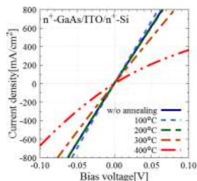
Fig.2 I-V characteristics of n<sup>+</sup>-GaAs/ITO/n<sup>+</sup>-Si junctions without and with annealing at 100, 200, 300 and 400 °C
