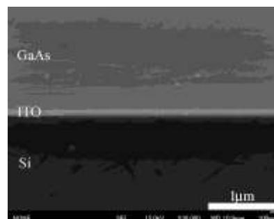
Fig.1 SEM image of GaAs/ITO/Si junctions
